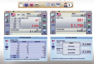
MIB-11V Currency Discriminator Model is equipped with userinterface allowing users to choose simple or detail count display screen as well as to change count from Black to Red large font. User can view Day Total and Grand Total - Print them or Clear.
